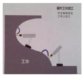
Ultra-large workpiece processing can be directly adsorbed on the workpiece surface, the position of the machine head can be arbitrarily adjusted.
