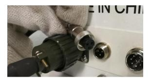
14. 8-pin head dual plug cable is for the rotary clamp accessory(optional), as shown below.
