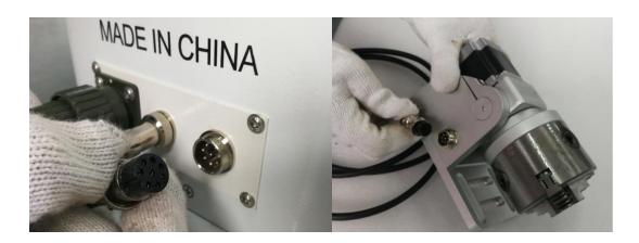
15. The industrial tablet power supply can be installed in two ways, ① Use the 2-pin dual plug connect the industrial tablet USB port with the top cover USB port, as shown below. ② Use the standard power supply cable, you can directly plug into the power outlet.
