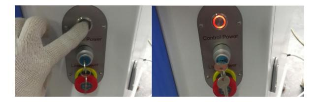
19. Under normal, not marking condition, the safety led light is green. When the machine is marking, the safety led light will turn to yellow, press the emergency stop switch, the safety led light will turn red and accompanied by high pitch noise.
