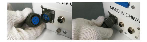
13. 3-pin head cable is for the footswitch, insert into the socket, rotating to lock-in position, as shown below.
