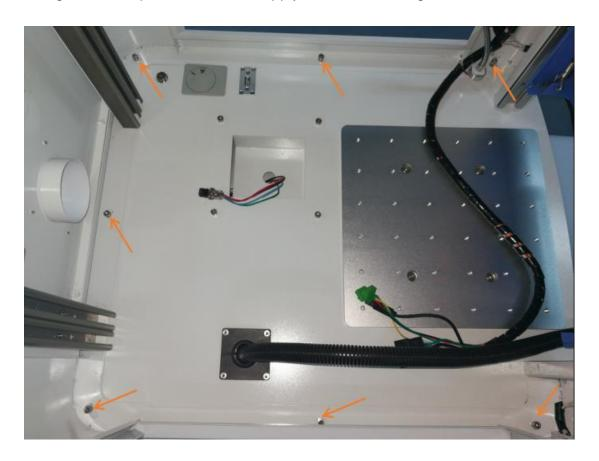
8. The green plug is the safety led light connector, and the big black one connects the button sets on the front panel of the top cover. The other small plug is for the USB cable communication.
