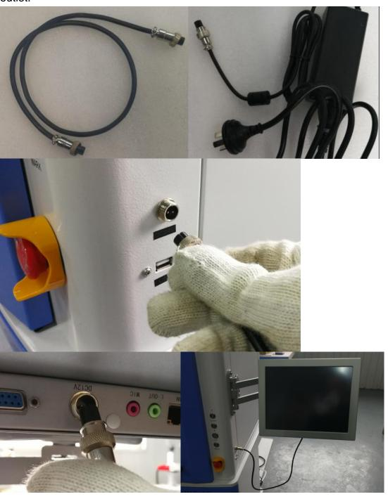
16. USB communication cable connection, connect the top cover USB port with industrial tablet USB port, as shown below.
