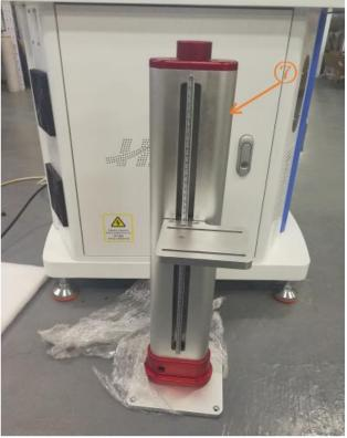
2. The seven screw holes on the supply unit table are fixed. Place the laser marking head as shown below.
